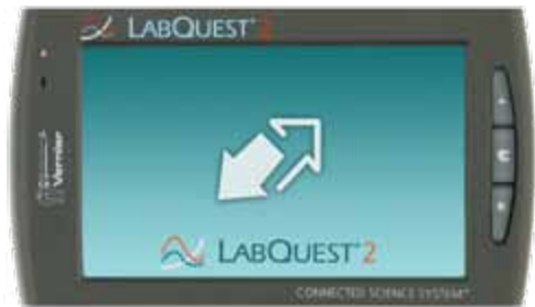
A double arrow indicates the computer is in control of LabQuest.
